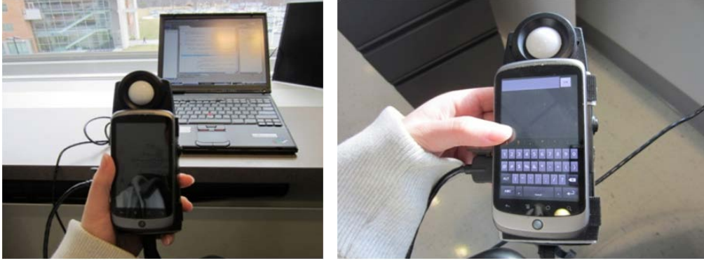
Figure 3: Experimental setup. The handheld device was attached to the face of the T-10 such that the sensor was able to capture illuminance readings of the background. The T-10 was connected to a laptop computer through a proprietary RS232 cable because due to Android OS limitations, the handheld devices were not able to directly interface with the T-10. The T-10 reading and writing program was run on the laptop so that it was able to read data from the T-10 and write measurements into a text file which was used for data analysis. A time stamp synchronized each user response from the DENOTE application with the exact illuminance measurement.
