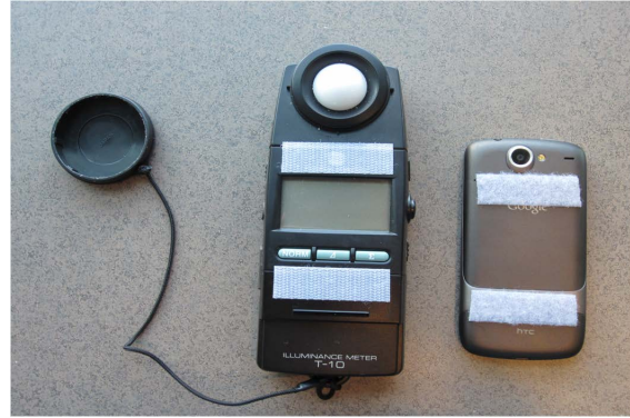
(b) Velcro was attached to both the T-10 illuminance meter and the mobile device.
